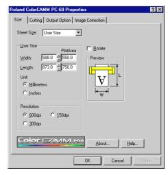
Set the [PlotArea]. We will devide the data into half so we will set the [Length] to the half of the size ((W)  $550 \times (L)$  750mm) of the original data ((W)  $550 \times (L)$  1500mm).
